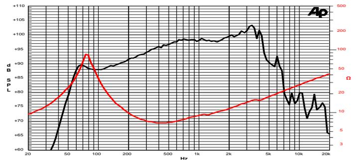
Frequency Response on 25 Lt @ 65 Hz Vented Box @ 1W, 1m
