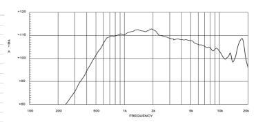
HD1480T MEASURED WITH 1W INPUT ON RATED IMPEDANCE AT 1M DISTANCE ON XR1464 HORN MOUTH AXIS
